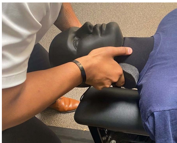
Figure 4 - Supine cervical adjustment on Human Analogue Mannequin (HAM™) with the Handheld Tri-Axial Load Cell at the doctor/patient interface to measure adjustment time parameters.
