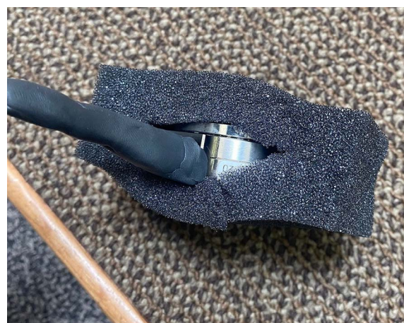
Figure 3 - Handheld Tri-Axial Load Cell by ATI Industrial Automation (model number FTIFPS1).
