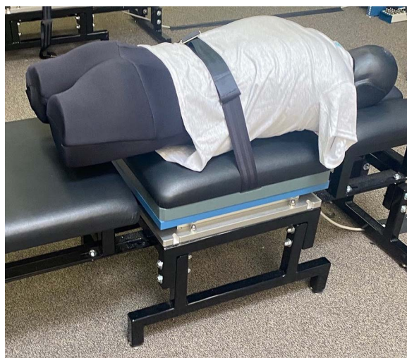
Figure 2 - Human Analogue Mannequin (HAM) secured on Force Sensing Table Technology (FSTT) version 1.9 (Canadian Memorial Chiropractic College, Toronto Canada) adjusting table with a seatbelt to minimize movement during adjustments.
