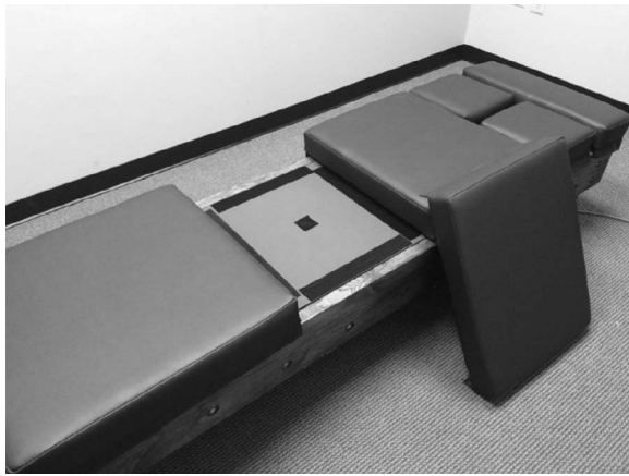
Figure 1 - A photograph of the force plate in the lumbar section of the adjusting table. The force plate is mounted on rails attached to the table sides and isolated from other sections of the table. Table padding is removable.
